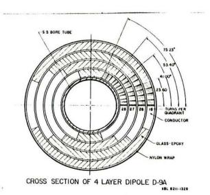
Fig. 1. Cross section of the D-9A Dipole.
