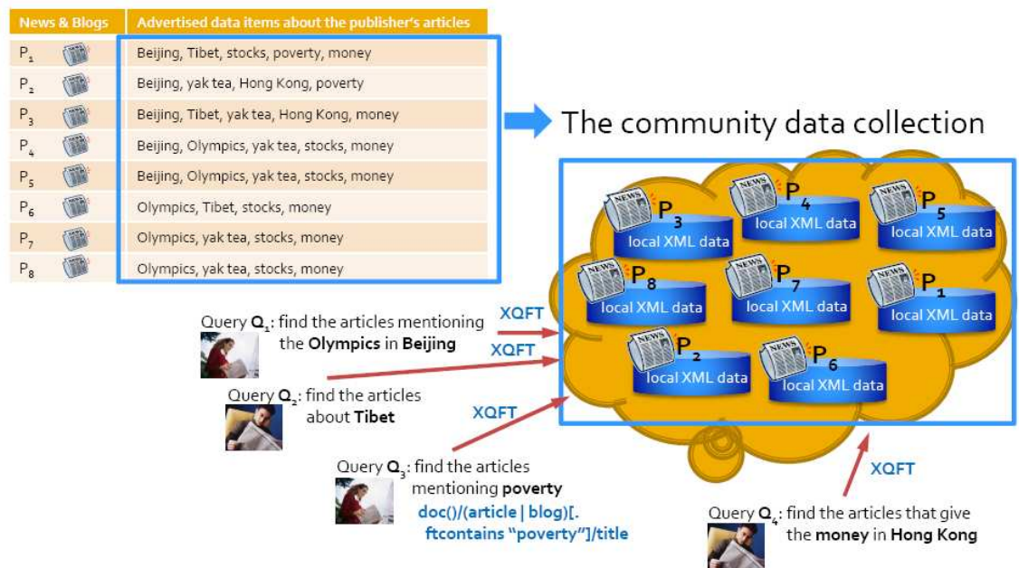
Figure 1.3: The community data: publishers advertise terms about their local data store, which is accessible via an XML-based full-text search interface
