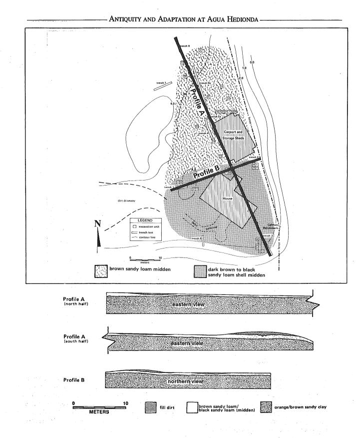
Figure 3.3. Site soil profile based on trench and excavation unit data.
