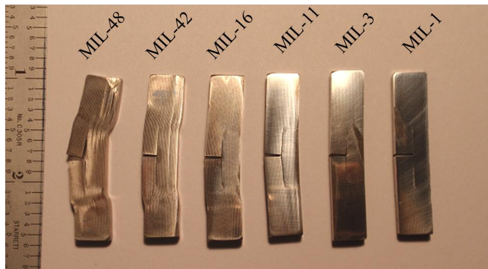
Figure 4.29 – Photograph of an arrester samples from each specimen after testing in quasi-static 4PB. Notice the lack of fracture in the notch direction.
