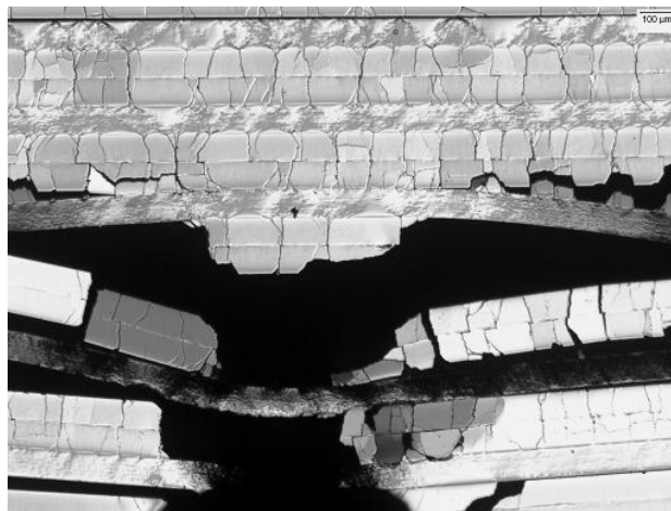
Figure 4.67– (a) High-speed camera images showing the failure of MIL-1 under dynamic 4PB. (b) Optical micrograph of the notch tip seen in (a) at 222 microseconds.
