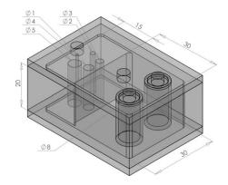
Figure 2.3: Schematic drawing of image the quality phantom used in some of the Genisys studies. All dimensions are in millimeters. Activity concentration within one of the large cylindrical chambers was approximately 5x that of the rectangular pool. The other large cylindrical chamber was filled with inactive saline. The five rods (varying in diameter between 1 mm and 5 mm) consisted of an activity concentration equal to that of the pool.
