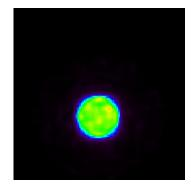
Figure 5.8: Example transaxial image of the spherical phantom scanned with the preclinical Genisys G4 scanner. The size of this slice is  $96 \times 96 (0.46 \text{ mm x } 0.46 \text{ mm})$ . The colorbar has been adjusted to accommodate the entire dynamic range of voxel values. No noticeable artifacts prevent calculation of the centroid.
