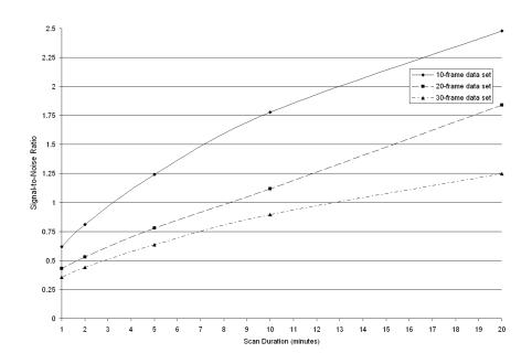
Figure 4.7: SNR calculated from PCA Genisys results shown in Figure 4.6. These curves indicate increasing benefit in SNR as activity is increased, regardless of the number of frames reconstructed. The total activity within the cylinder was approximately 40 µCi for all data sets.
