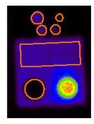
Figure 2.4: Coronal image of phantom with ROIs drawn to segment the various sections. The hot cylindrical chamber is on the lower right. The rectangular pool physically encompasses both cylindrical chambers, but its ROI is drawn to prevent contamination from the rods and hot chamber. Four of the five rods are visible in the upper central portion.
