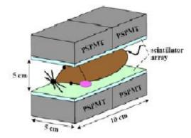
Figure 2.1: Dual head configuration of the Genisys microPET system. The lack of detectors in the sagittal direction gives rise to the image artifacts (i.e. "bowtie" artifact) which severely limits image quality. Due to the isotropic nature of radiation, detection must be performed with a full tomographic system in order to obtain statistically complete information.
