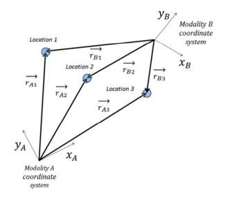
Figure 5.3: Illustration of calibration data used by Horn's method for computing the rigid body transformation. Three random points are chosen to be localized within each FOV. The points themselves are stationary relative to the bed. Mathematically, at least three noncollinear points are needed to compute a transformation.
