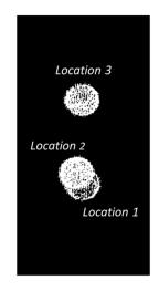
Figure 5.9: Fusion of three separate microCT coronal images of the spherical phantom. The phantom was repositioned in between scans. Centroids of each sphere were computed individually. These images were used to compute the coregistration transformation between the microCT and the Inveon microPET systems.
