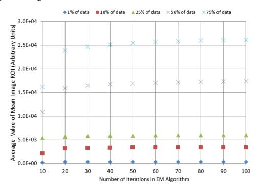
Figure 2.9: Average pool ROI values derived from mean images. Average values are relatively consistent after ~40 iterations regardless of how much data is used.
