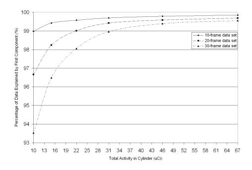
Figure 4.8: Percentage of Inveon data explained by the first component computed for each set using a total scan duration of 20 minutes for each set. These curves demonstrate "diminishing returns" in terms of percentage explained as scan duration is increased.
