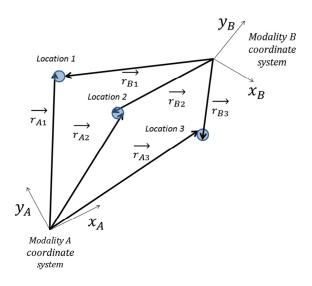
Figure 5.4: Graphical illustration of calibration data used for computing the rigid body transformation. Unlike what is shown in Figure 5.3, the same three points are not localized by both systems. The error in the measurement will degrade the accuracy of the coregistration.
