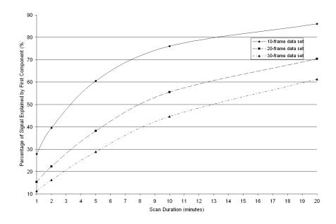
Figure 4.6: Percentage of Genisys data explained by the first component computed for each set using a total scan duration of 20 minutes for each set. These curves demonstrate "diminishing returns" in terms of percentage explained as scan duration is increased.
