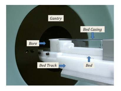
Figure 5.2: Bed apparatus used within the Siemens Inveon preclinical PET system. For visual clarity, no subject is shown, and the bed is only partially inserted into the bore. In practice, the bed is fully inserted into the bore so that the subject within the bed lies within the FOV. Identical bed tracks are fitted to each imaging system allowing the bed to be inserted into each system without having to reposition the subject between scans.
