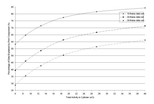
Figure 4.10: Percentage of Genisys data explained by the first component computed for each data set using a total scan duration of 20 minutes for each set. These curves demonstrate "diminishing returns" in terms of percentage explained as scan duration is increased.
