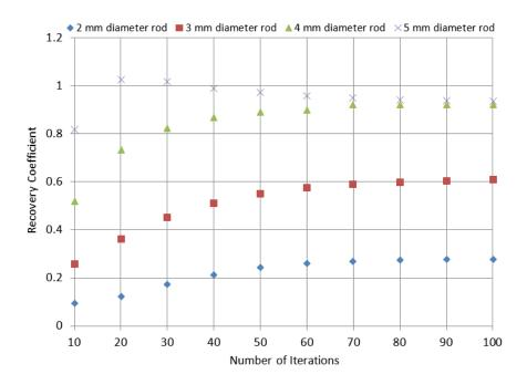
Figure 2.14: Recovery coefficients of rods using 10% of data. The 1 mm diameter rod was not visible in the final image. Most coefficients are less than 1. However, coefficients greater than 1 are possible due to spillover of activity from the periphery of the rod into the centroid.
