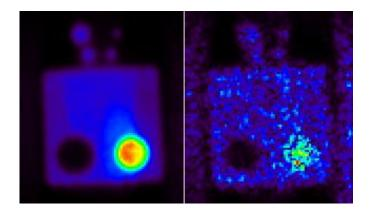
Figure 2.6: Mean image (left) and standard deviation image (right) computed for the phantom using four subset images each created with 1% of the data. One of the four images is shown in Figure 2.5.
