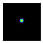
Figure 5.7: Example transaxial image of the spherical phantom scanned with the Inveon preclinical PET scanner. The size of this slice is  $128 \times 128$  (0.86 mm x 0.86 mm). The colorbar has been adjusted to accommodate the entire dynamic range of voxel values. No noticeable artifacts prevent calculation of the centroid.
