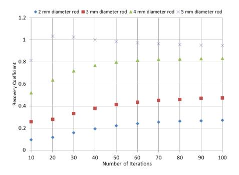
Figure 2.15: Recovery coefficients of rods using 25% of data. The 1 mm diameter rod was not visible in the final image. Most coefficients are less than 1. However, coefficients greater than 1 are possible due to spill over of activity from the periphery of the rod into the centroid.
