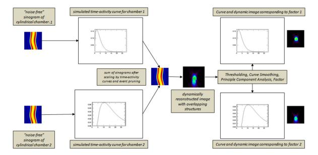
Figure 3.7: Diagram illustrating the overall method used in the production of the synthetic images. Two different synthetic TACs are used to scale the sinograms representing each of the
