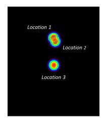
Figure 5.10: Fusion of three separate Inveon coronal images of the spherical phantom. The phantom was repositioned in between scans. The locations indicated correspond to those in Figure 5.9. Centroids of each sphere were computed individually.
