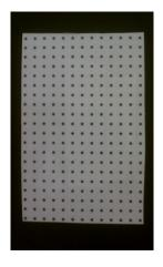
Figure 6.3: Photograph of the printed grid consisting of 260 dots. Each dot is 1.0 mm in diameter, and spaced 5.0 mm away from adjacent dots. The grid was laminated in order to increase rigidity. After imaging of the grid, the centroid locations of each dot within in the FOV
