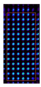
Figure 6.5: Coronal slice used in spatial linearity measurement taken from the Genisys image of the second grid using  $\emptyset = 2.0$  mm dots with 6.0 mm grid spacing. The slice is 80 x 176 voxels (0.55 mm x 0.55 mm). The dots near the edge of the FOV exhibit significant distortion and, therefore, were excluded from the centroid analysis. The 84 dots within the rectangular ROI were used in the analysis.
