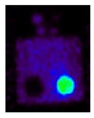
Figure 2.5: Coronal image of phantom using 1% of the data used to create the image shown in Figure 2.4. The same number of iterations (50) and smoothing filter was used as that for Figure 2.4. Four of these subsampled images were created independently for each percentage and each iteration.
