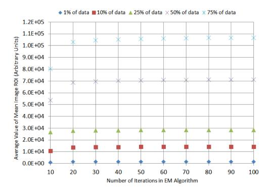
Figure 2.7: Average hot chamber ROI values derived from mean images. Regardless of how much of the original data set was used, there is relatively little change after ~30 iterations.
