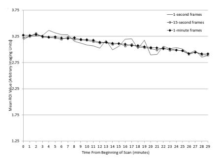
Figure 3.4: <sup>18</sup>F decay curves measured from the raw dynamic images pertaining to the <sup>18</sup>F ROI shown in Figure 3.2. The 1-minute data set makes full use of all acquired data and is, therefore, the least noisy. The scaling is set to match that of Figure 3.3 for visual comparative purposes.
