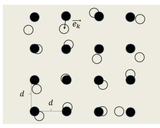
Figure 6.1: Graphical illustration of measuring the spatial linearity of an imaging system. Positions of the regularly-spaced physical points are shown in solid black; their corresponding measured positions within the image are shown as empty circles. The error between each grid point and its corresponding image is measured as a vector  $\vec{e_k}$ . All adjacent grid points are spaced by a fixed distance *d*. Although the concept is applicable in 3D, it is shown in 2D for visual clarity.
