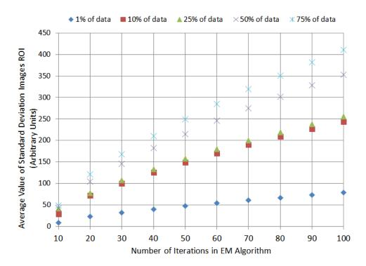
Figure 2.10: Average pool ROI values derived from standard deviation images. . It is clear that these values increase steadily with iterations, especially for the sets with a higher percentage of the original data.
