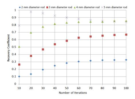
Figure 2.13: Recovery coefficients of rods using 1% of data. The 1 mm diameter rod was not visible in the final image. All recovery coefficients are less than 1, indicating that the spillover effect is dominant regardless of the number of iterations used.
