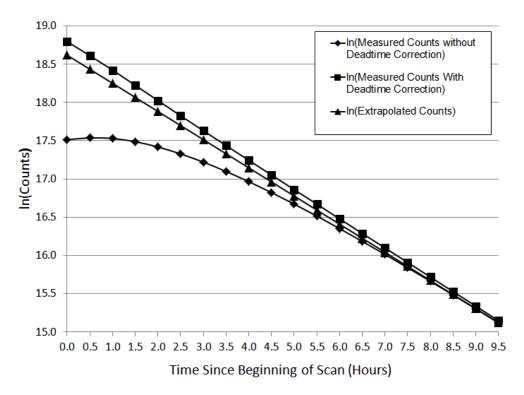
Figure 2.19: Semi-logarithmic plot indicating the measured counts without deadtime correction and the extrapolated true counts. The measured counts with deadtime correction are shown only for visual comparison; it was not used within the analysis.
