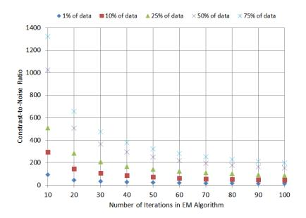
Figure 2.11: Contrast-to-noise ratio measured using ROIs from hot chamber and pool. Contrast itself was found to be slightly lower than expected, but relatively constant regardless of the
