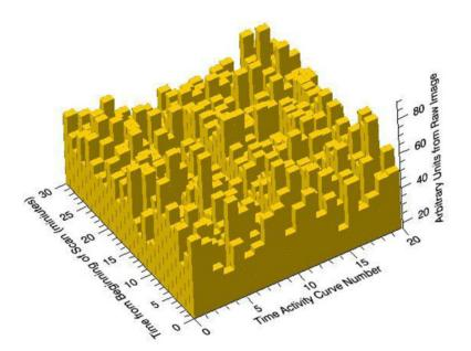
Figure 3.6: Example of voxel-based TACs from dynamic image. TACs derived from the <sup>18</sup>F ROI shown in Figure 3.2. The TACs exhibit signs of random noise, but not natural decay due to the relatively long half-life of <sup>18</sup>F (109.8 minutes). The natural decay of <sup>11</sup>C shown in Figure 3.5 is more apparent. For visual clarity, only 20 of the 665 TACs selected from the <sup>18</sup>F ROI are shown here.
