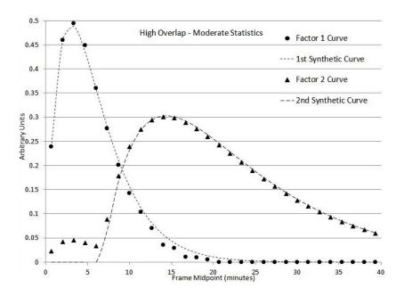
Figure 3.10: Results for the "high overlap" and "moderate statistics" data sets from the semiquantitative study shown in Figure 3.7. All curves have been normalized to unity using the Euclidean norm.
