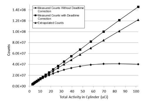
Figure 2.20: Counts acquired as a function of activity within the Genisys system. The activity indicated is based on the half-life of <sup>18</sup>F (109.8 minutes) and the initial activity (102  $\mu$ Ci) as measured by a dose calibrator prior to the scan. The true counts were extrapolated from the region of lowest activity where deadtime is the least intrusive. The measured counts with deadtime correction are shown only for visual comparison; it was not used within the analysis.
