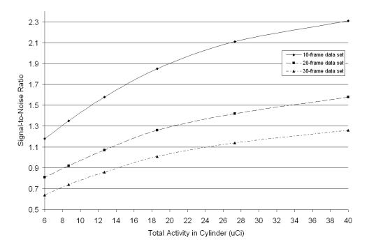
Figure 4.11: SNR calculated from PCA Genisys results shown in Figure 4.10. These curves indicate increasing benefit in SNR as activity is increased, regardless of the number of frames reconstructed.
