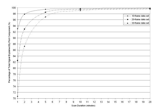
Figure 4.4: Percentage of Inveon data explained by the first component computed for each set using a total activity of approximately 80  $\mu$ Ci. These curves demonstrate "diminishing returns" in terms of percentage explained as scan duration is increased.
