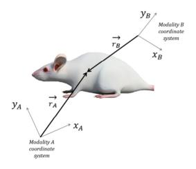
Figure 5.1: Graphical illustration of the rigid body coregistration problem. The coordinate systems of two modalities, A and B, are translated and rotated arbitrarily with respect to one another. The rigid body coregistration problem consists of finding the optimal rotation and translation such that alignment between the two systems is as close as possible. For simplicity, only a 2-dimensional view is shown. In practice, the imaging and coregistration are performed in all three dimensions.
