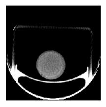
Figure 5.5: Example transaxial image of sphere scanned within the microCT scanner. The size of this slice is  $256 \times 256 (0.2 \text{ mm x } 0.2 \text{ mm})$ . The centroid of this sphere is the quantity of interest, but the nonzero voxels of the bed and nonuniformity within the sphere precludes this. Additional image processing must be performed before the geometrical centroid can be calculated.
