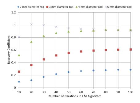
Figure 2.16: Recovery coefficients of rods using 50% of data. The 1 mm diameter rod was not visible in the final image. Most coefficients are less than 1. However, coefficients greater than 1 are possible due to spillover of activity from the periphery of the rod into the centroid.
