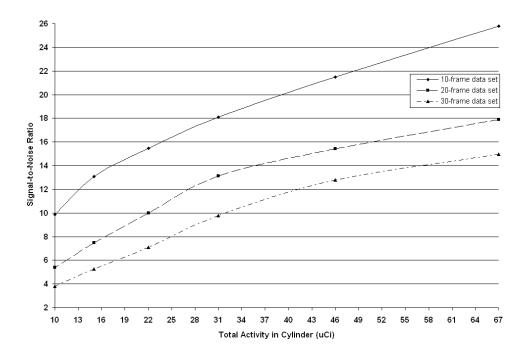
Figure 4.9: SNR calculated from PCA Inveon results shown in Figure 4.8. These curves indicate increasing benefit in SNR as activity is increased, regardless of the number of frames reconstructed.
