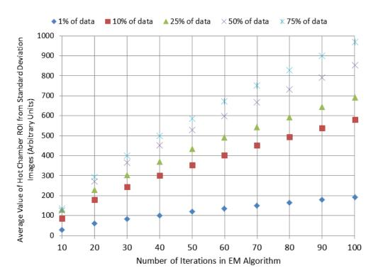
Figure 2.8: Average hot chamber ROI values derived from the standard deviation images. It is clear that these values increase steadily with iterations, especially for the sets with a higher percentage of the original data.
