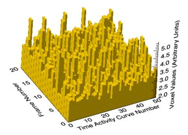
Figure 4.3: A subset of nonzero TACs taken from an Inveon 5-minute acquisition reconstructed into 20 frames using the protocol of the first study. Most data sets used in these studies consist of  $\sim$ 2000 nonzero TACs; only the 50 TACs with the largest norms have been shown here for visual clarity.
