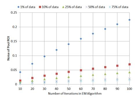
Figure 2.12: Relative noise derived from pool ROI values. The relative noise increases in a linear fashion with the number of iterations, regardless of how much of the original data set was used.
