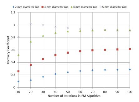
Figure 2.17: Recovery coefficient of rods using 75% of data. The 1 mm diameter rod was not visible in the final image. Most coefficients are less than 1. However, coefficients greater than 1 are possible due to spillover of activity from the periphery of the rod into the centroid.
