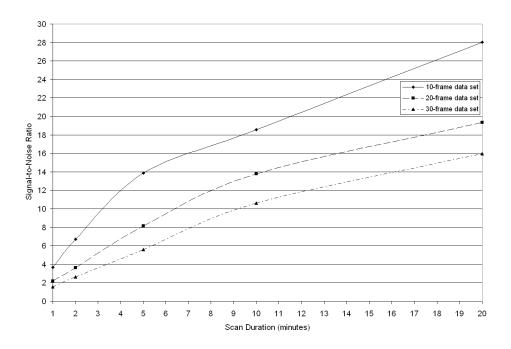
Figure 4.5: SNR calculated from PCA Inveon results shown in Figure 4.4. These curves indicate increasing benefit in SNR as scan duration is increased, regardless of the number of frames reconstructed.
