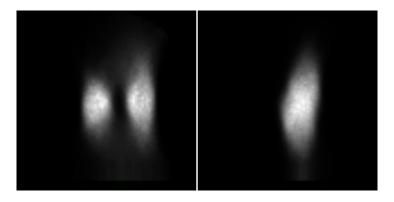
Figure 3.1: Transaxial slice of horizontally (left) and vertically (right) aligned chambers of approximately equal activity. Due to the limited angle tomography, clear separation is only possible when the sources are horizontal relative to each other.
