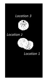
Figure 5.11: Fusion of three separate microCT coronal images of the spherical phantom. The phantom was repositioned in between scans. Centroids of each sphere were computed individually. These images were used to compute the coregistration transformation between the microCT and the Genisys G4 microPET systems.
