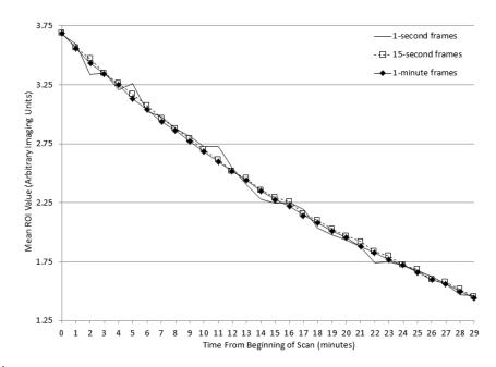
Figure 3.3: <sup>11</sup>C decay curves measured from the raw dynamic images pertaining to the <sup>11</sup>C ROI shown in Figure 3.2. The 1-minute data set makes full use of all acquired data and is, therefore, the least noisy.
