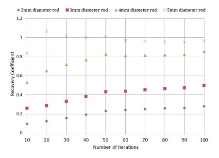
Figure 2.18: Recovery coefficients of rods using 100% of data. The 1 mm diameter rod was not visible in the final image. Most coefficients are less than 1. However, coefficients greater than 1 are possible due to spillover of activity from the periphery of the rod into the centroid. There appears to be slightly more fluctuation in the coefficients when using this complete data set compared to the randomly selected subsets.
