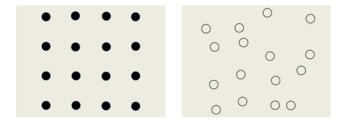
Figure 6.2: The synthetic grid composed of points with consistent grid spacing d is shown on the left. The image obtained from measured positions of these dots in shown on the right. The spatial linearity measurement shown in Figure 6.1 can be obtained by a rigid coregistration between this synthetic grid and the measured image.
