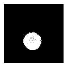
Figure 5.6: Cropping and thresholding applied to the sphere shown in Figure 5.5. All voxels which lie outside the sphere are set to have a value of zero. Most voxels within the sphere have a value of one, but a negligible few a value of zero due to the presence of voxel values below zero in the original image.
