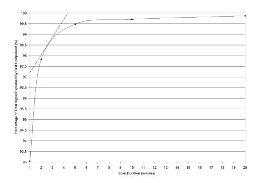
Figure 4.12: Example of finding the optimal point defined as the point of the curve at which the tangent slope (i.e. derivative) has a value of 1/min. The curve shown is the 10-frame data set rescaled from that in Figure 4.4. The 20-frame and 30-frame data sets have not been shown for visual clarity. The optimal point for this particular set occurs at a scan duration of ~2.5 minutes.
