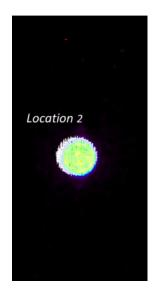
Figure 5.17: Coregistered coronal images of spherical phantom within the microCT and Genisys G4 at location 2. The sphere at location 2 in Figure 5.12 has been transformed to coincide with the sphere at location 2 in Figure 5.11.
