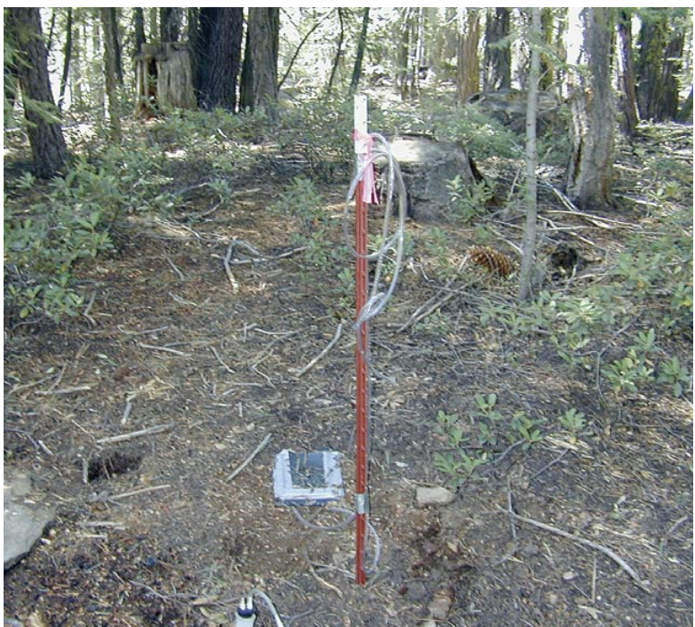
Data from runoff collectors, above, shows that runoff from overland/litter interflow seeps downslope through the organic surface layers during rainfall and snowmelt, never gaining enough momentum to cause physical disturbance.
