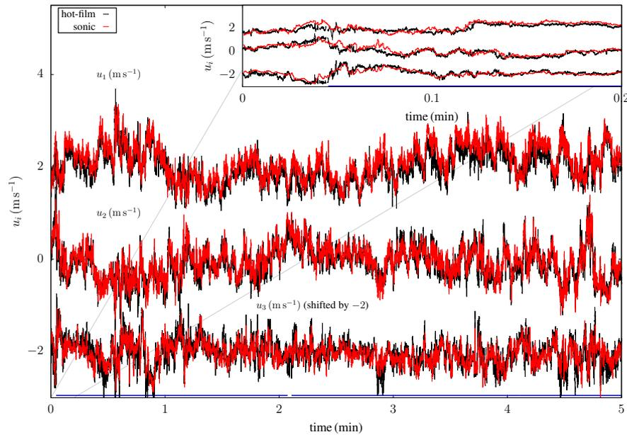
**Fig. 4** Sample of velocity time series from sonic (red) and hot-film (black) anemometers, starting at June 10 03:30h local time. Inset is a closer look into the first 12 seconds. Blue lines at the bottom indicate the 2-min subblocks without data gaps for this sample.
