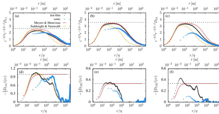
**Fig. 9** Nondimensionalized second- (upper panels) and third- (lower panels) order structure functions ((a,d) streamwise, (b,e) spanwise, (c,f) vertical). Hot-film/sonic anemometers data as grey/blue crosses, in addition to Meyers and Meneveau (2008)’s model and Saddoughi and Veeravalli (1994)’s data in red/yellow lines. The dashed black horizontal lines correspond to the theoretically predicted values for inertial range.
