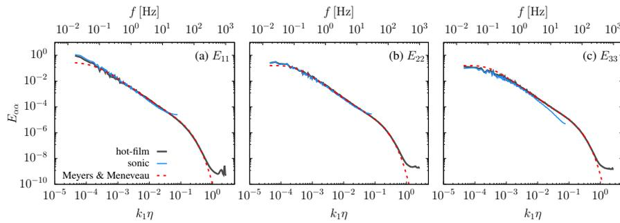
**Fig. 5** One-dimensional spectra for the (a) streamwise, (b) spanwise and (c) vertical velocities as a function of the streamwise nondimensional wavenumber and frequency. Spectra were smoothed using bin averages in log scale, and Taylor’s frozen turbulence hypothesis was used. Hot-film (grey) and sonic (blue) anemometers data, in addition to Meyers and Meneveau (2008)’s model (dashed red lines).
