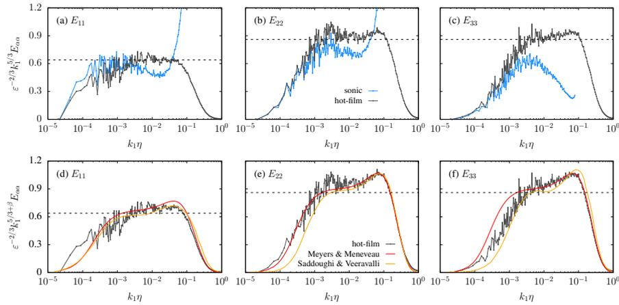
**Fig. 7** Compensated one-dimensional spectra of (a,d) streamwise, (b,e) spanwise, (c,f) vertical velocities as a function of the nondimensional wavenumber. Hot-film/sonic data in grey/blue lines, Meyers and Meneveau (2008)'s model and Saddoughi and Veeravalli (1994)'s data in red/yellow lines. The dashed black horizontal lines correspond to the theoretically predicted values for the inertial range.
