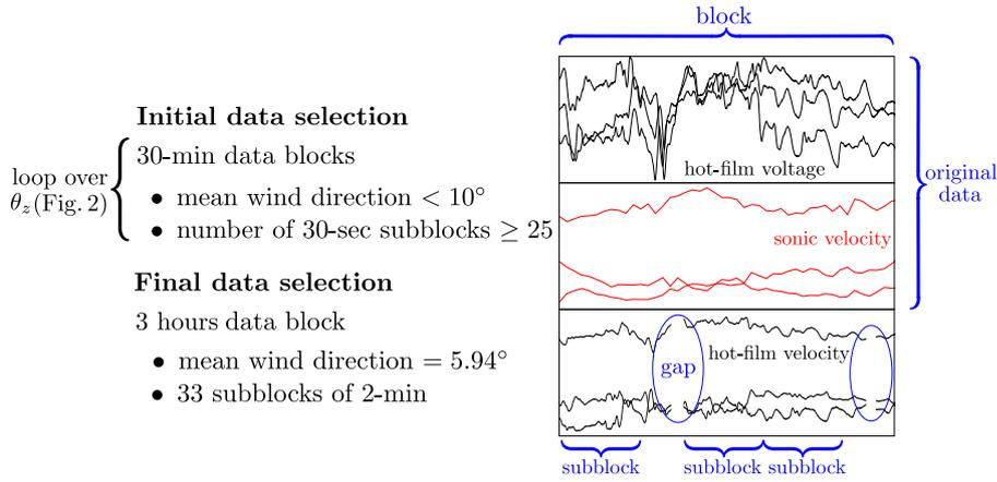
**Fig. 12** Summary of data selection and illustration of the blocks and subblocks used in this study. While the block consisted of a fixed period in the original data (hotfilm voltage and sonic velocity, 30-min and 3-hours long), the subblocks were formed in the final hot-film velocity series by selecting consecutive periods without gaps.
