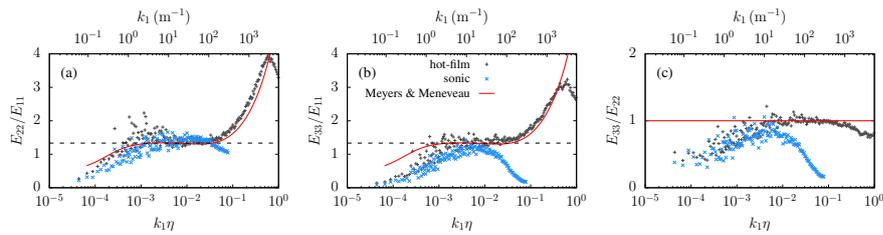
**Fig. 8** Ratios of the one-dimensional spectra. Hot-film/sonic anemometers data in grey/blue crosses, in addition to Meyers and Meneveau (2008)’s model (red lines). The dashed black horizontal lines correspond to the theoretically predicted  $4/3$  value for the inertial range.
