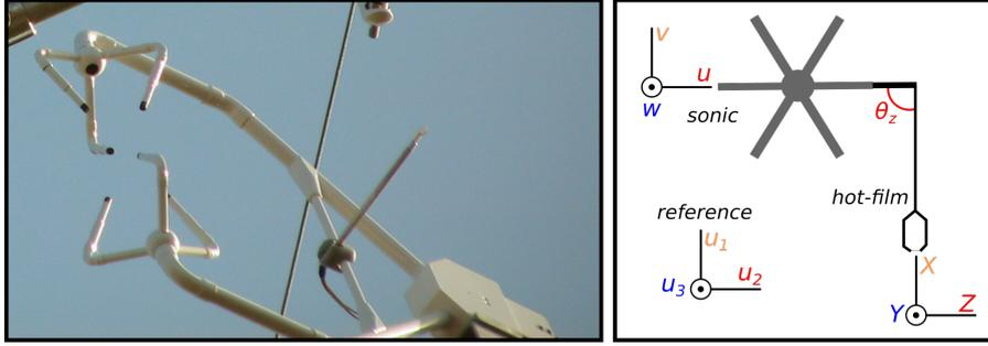
**Fig. 1** Left: picture of the sonic and hot-film sensors in the field (hot-film attached to the vertical support of the sonic arms in a  $90^\circ$  angle). Right: top view of the coordinate system of the sonic  $\langle u, v, w \rangle$  (pointing westward) and hot-film  $\langle X, Y, Z \rangle$  (pointing southward). We define the reference coordinate system as  $\langle u_1, u_3, u_2 \rangle$  and redefine the sonic and hot-film data accordingly.
