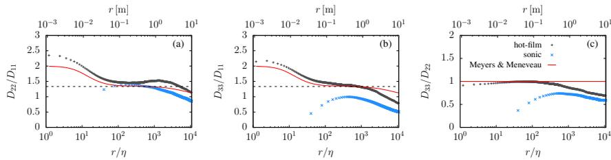
**Fig. 10** Ratios of the second-order structure functions. Hot-film (grey) and sonic (blue) anemometers data, in addition to Meyers and Meneveau (2008)'s model (red lines). The dashed black horizontal lines correspond to the theoretically predicted values for the inertial range.
