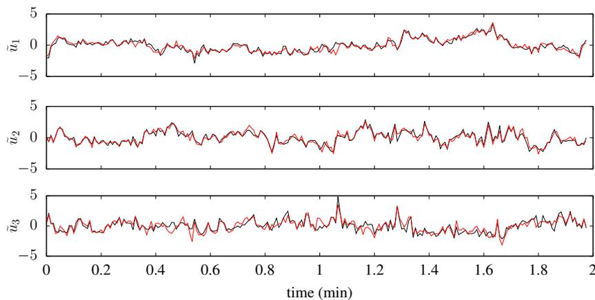
**Fig. 14** Time series of the filtered and rescaled velocity vector (filtered at the 2 Hz frequency, rescaled by their mean and standard deviation of the subblock) of the hot-film (black) and sonic (red) data, for the last 2-min block.
