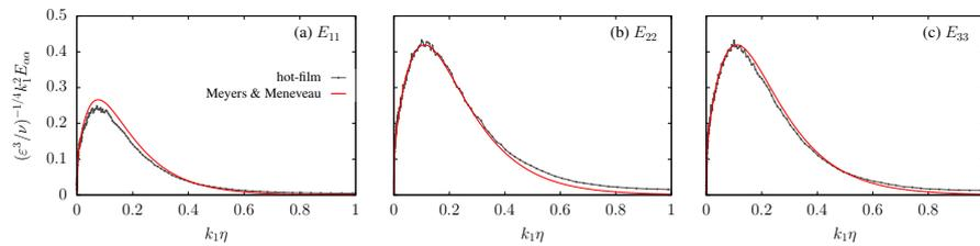
**Fig. 6** Dissipation spectra for the (a) streamwise, (b) spanwise and (c) vertical velocities as a function of the nondimensional wavenumber. Hot-film data in grey and Meyers and Meneveau (2008)’s model in red. The mean dissipation rate was estimated as the average of the integrals of these three data curves (Eq. (5)).
