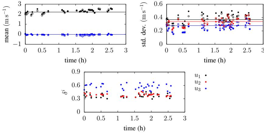
**Fig. 13** Block average (3 hours, solid lines) versus subblocks statistics (2-min, circles). Filled (open) circles are sonic (hot-film) data. Mean (top left), standard deviation (top right) and delta parameter (bottom) of the streamwise (black), spanwise (red) and vertical (blue) velocities.
