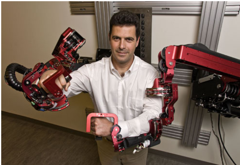
Figure 1.2: EXO-UL7, a dual arm exoskeleton with seven DOFs in each arm. This system exhibits kinematic redundancy identical to the human arm.
