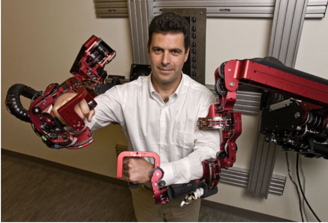
Figure 4.1: The upper limb exoskeleton with seven DOFs, supporting 99% of the range of motion required to preform daily activities.
