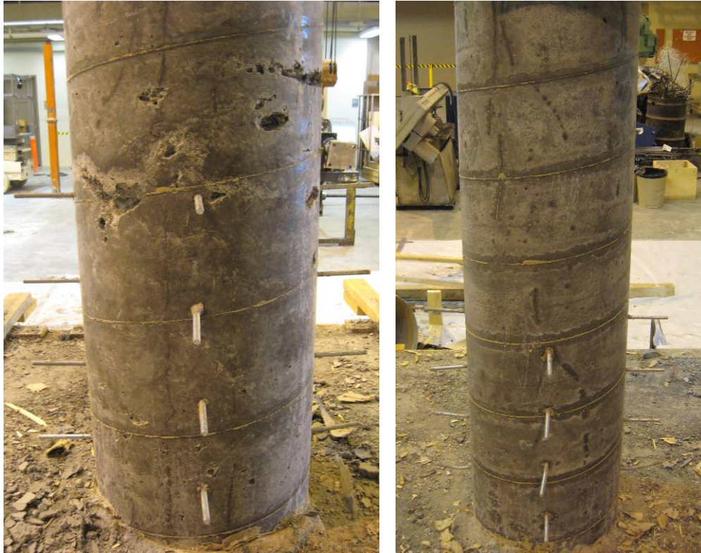
Figure B-12 Specimens after the removal of the forms (a) S1 column; (b) S2 column
