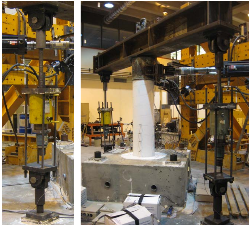
Figure B-19 Vertical load setup including spreader beam, top and bottom spherical clevises, prestressed rods, and hydraulic jacks: (a) Detail; (b) Global view
