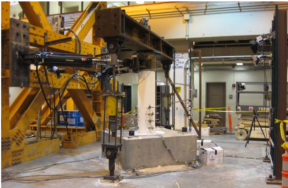
Figure B-14 Final setup of S1 and S2 FRC column specimens
