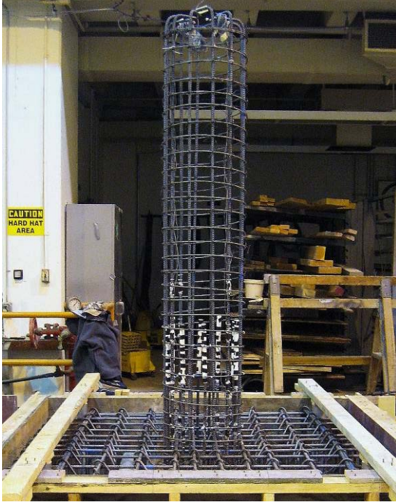
Figure B-3 Column cages with strain gages on longitudinal and transverse reinforcement and unbonded PVC tubes: (a) specimen S1; (b) specimen S2
