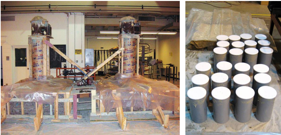
Figure B-11 (a) Curing of column specimens; (b) Curing of plain concrete and fiber-reinforced concrete cylinders and beams
