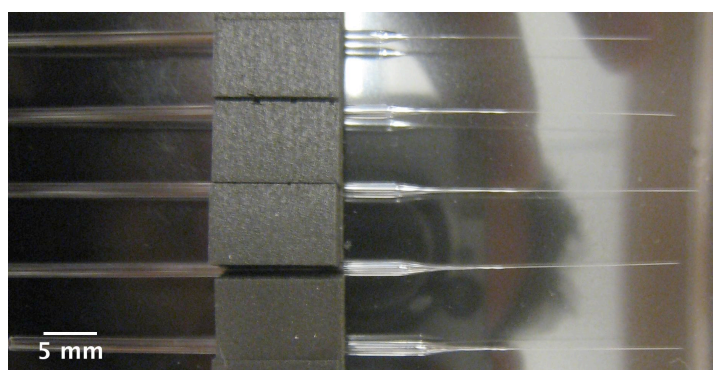
Figure 4. Glass capillaries pulled with a pipette puller modified to allow for longer pulling lengths.
