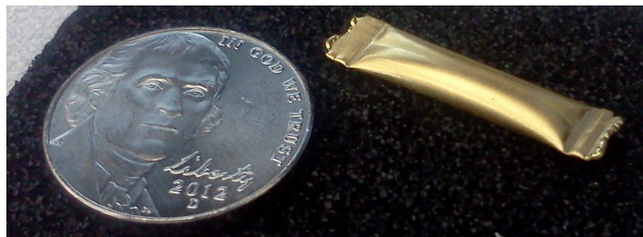
Figure 2.26. A welded gold capsule shown with a U.S. nickel as a scale reference. The capsule is filled with salt water brine and a 4x4 mm 4H-SiC die.
