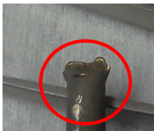
Figure 2.27. This gold capsule burst at the crimp location. The gold is coated with an ethylene glycol residue used in the water pressure lines in the test vessels.
