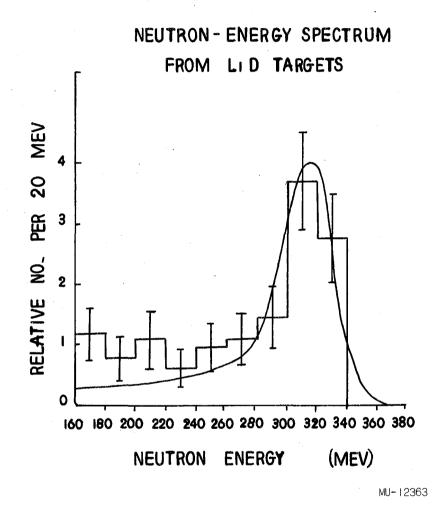
Fig. 1. The uniform curve represents the neutron spectrum obtained from a 0.5-inch LiD target by W. P. Ball. Superimposed on this curve is a histogram of the neutron-energy spectrum obtained from a 1-inch LiD target used in the xenon experiment.
