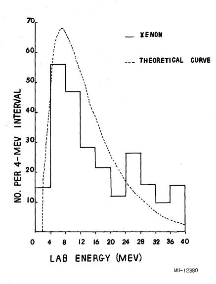
Fig. 22. The energy spectrum of all particles of unit charge emitted from Xe. The curve represented by the broken line is the theoretical curve of LeCouteur, which includes the effect of the decreased Coulomb barrier due to excitation of the nucleus.
