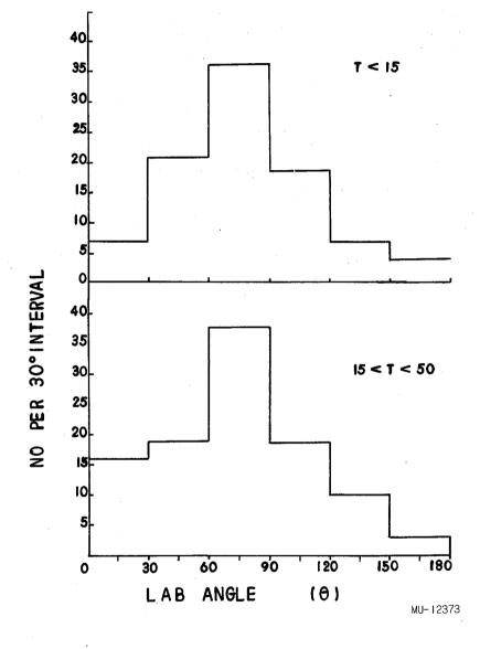
Fig. 15. The angular distribution (in the laboratory system) of protons emitted from xenon occurring in events not associated with mesons. Upper: the energies are less than 15 Mev. Lower: the energies of the protons are between 15 and 50 Mev.
