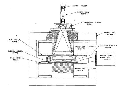
Fig. 3. The cloud chamber and magnet.
