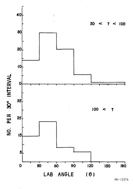
Fig. 16. The angular distribution (in the laboratory system) of protons emitted from xenon occurring in events not associated with mesons. Upper: the energies of the protons are between 50 and 100 Mev. Lower: energies exceed 100 Mev.
