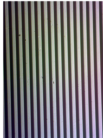
(b) calibrated Ronchi ruling, 1 bar = 25\ \mu\text{m}
