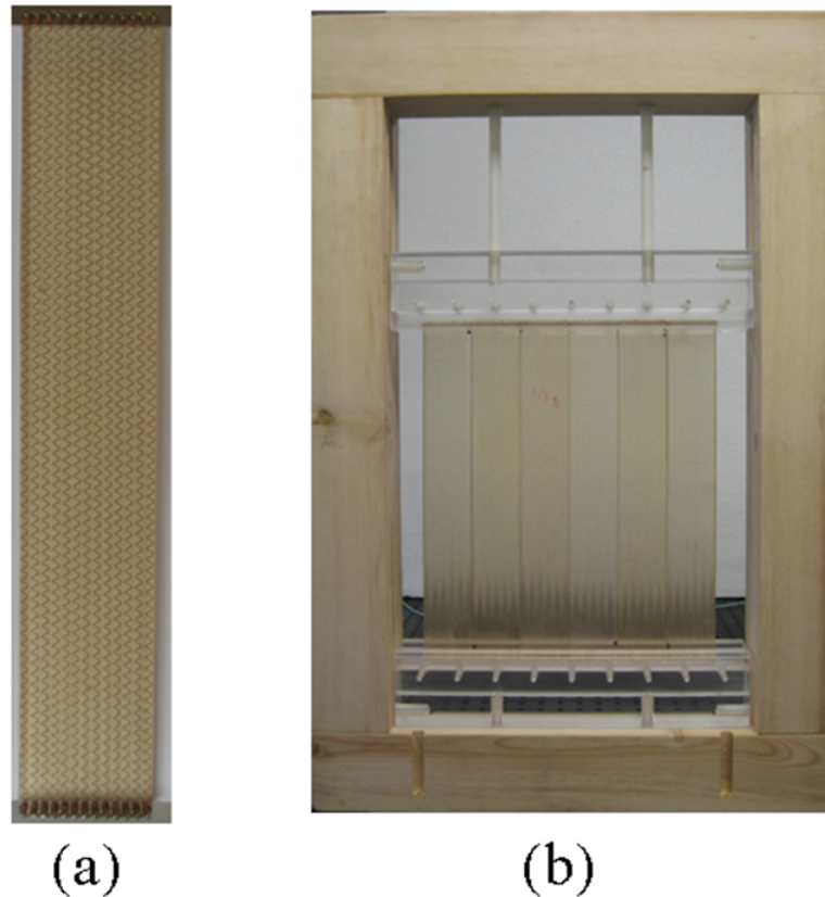
Figure 4.9: Sample used in the mechanical and EM tests. (a) One unit consists of 13 coils. (b) 6 units in the test frame for a total area of 310 mm x 310 mm.
