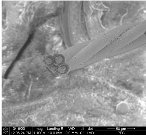
Figure 1.11: Scanning electron microscope image of a tetrode shaft and tip. Four 13\ \mu\text{m} nichrome electrodes are twisted together to produce one tetrode. The insulation is fused with a heat gun and the conducting tips are exposed.
