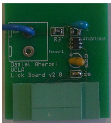
Figure 2.16: Capacitive touch sensor for detection of reward tube checking. (Left) Capacitive touch sensor circuit board. (Right) Schematic of capacitive touch circuit.
