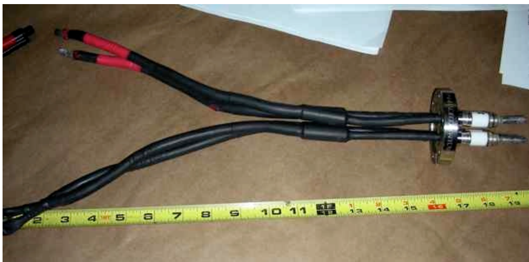
Figure 9. Two Pairs of Flexible Copper Leads Attached to a Vacuum Tight Feed-through for Magnet 2A
