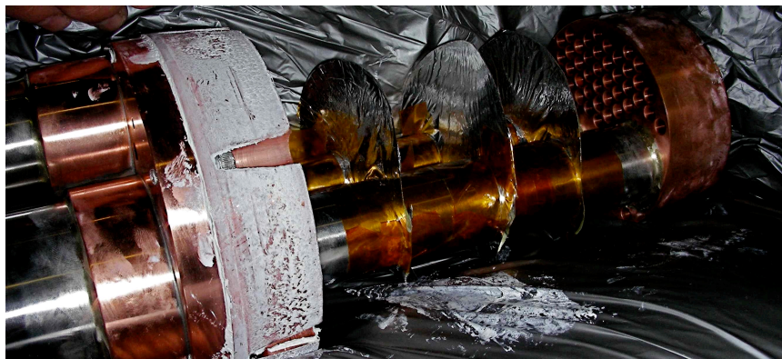
Figure 13. First-stage pressed tapered fit with vacuum grease (left), and second stage condenser (right).
