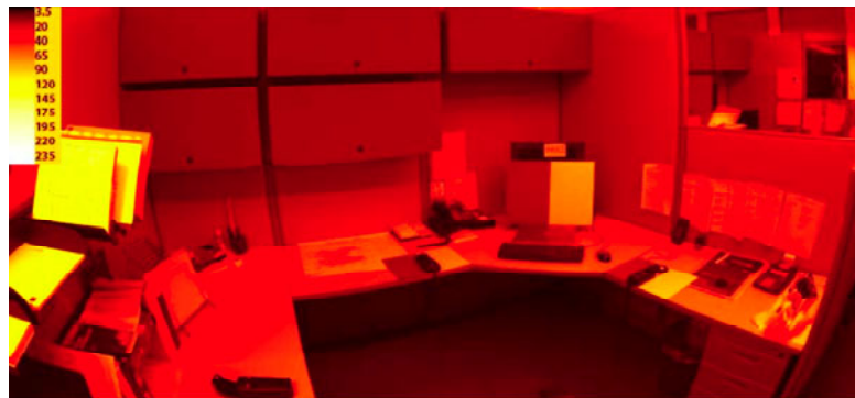
Figure 7. False Color Map Showing Measured Luminance Distribution of Uncluttered Cubicle Lit with the Base Fixture
