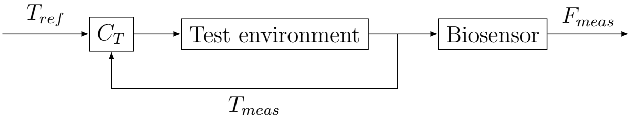
Figure 3.1: Open-loop characterization of the biosensor system’s response to ambient temperature profiles. The temperature profiles is defined by T_{ref} = T_{ref}(t) and regulated by the (inner loop) temperature control system C_T .
