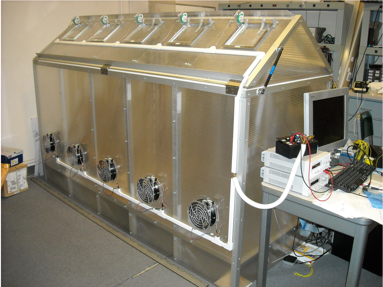
Figure 3.6: The test greenhouse, clearly showing five independently actuated bays. At the bottom of each bay is a sealable fan corresponding to the control input u_f in Figure 3.7. At the top of each bay, on the near pitch of the roof, is an actuated vent corresponding to the control input u_v in Figure 3.7. The cRIO chassis and interface computer shown at right.
