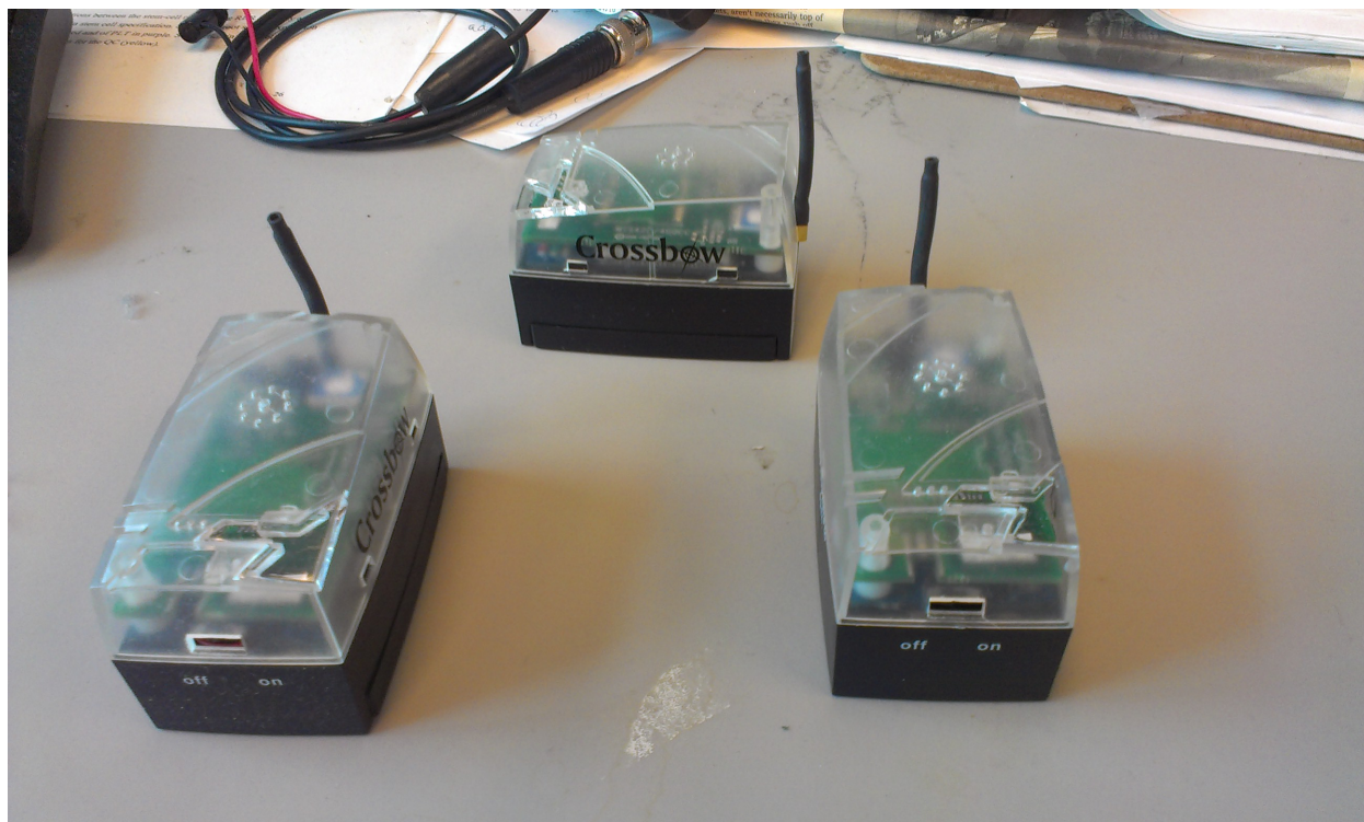
Figure 3.3: Three Crossbox MTS-420 wireless sensor nodes.
