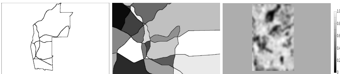
Figure 4.3: The image on the left shows the location of Hollenbeck in the N \times M environment grid. The semi-permeable boundaries encoded in the model are displayed in the center image. The shades of gray of this image are used to distinguish among regions. On the right, we used a Weighted H^1 Maximum Penalized Likelihood Estimation method with a road map as the initial data to approximate the road density of Hollenbeck [121]. The scale, seen on the far right, gives the approximated road density intensity. Light shades of gray correspond to high density values near one and dark shades correspond to low densities near zero.
