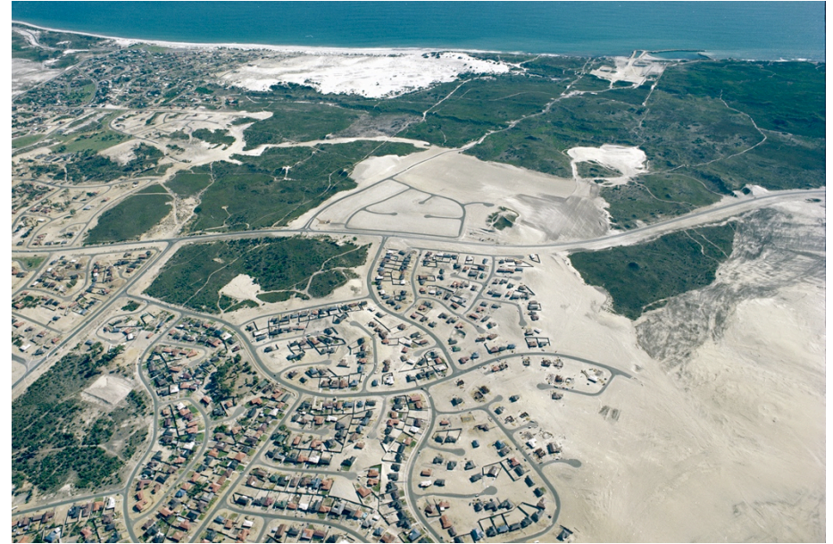
Figure 15: 1980 oblique aerial view over Heathridge and Ocean Reef. Total clearance and smoothing of the site without retaining walls prior to construction of streets and houses is evident (courtesy of State Library of Western Australia).
