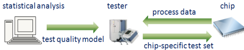
Figure 5.2 Proposed process-aware delay test flow
