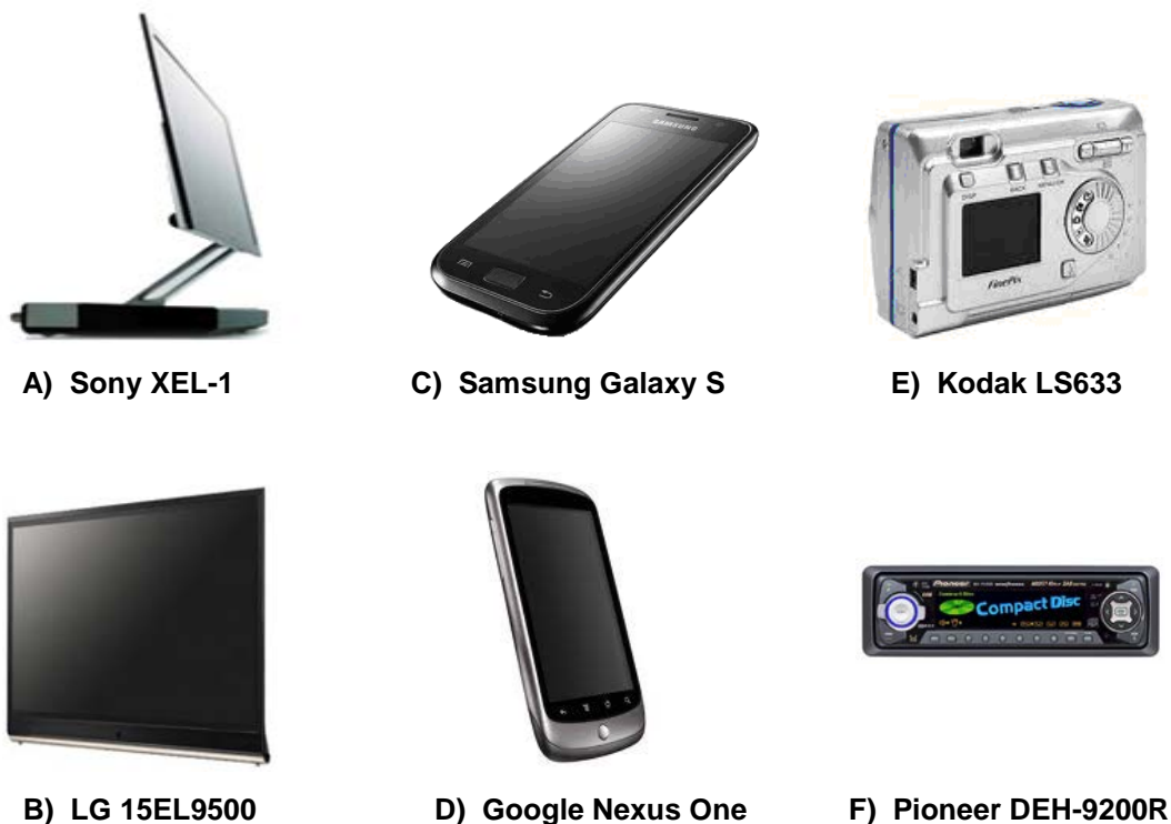
Figure 1.2: Commercialized OLED devices: OLED TVs, (A) Sony XEL-1 and (B) LG 15EL9500; AMOLED mobile phones, (C) Samsung Galaxy S and (D) Google Nexus One; digital camera, Kodak LS633; car stereo, Pioneer DEH-9200R.
