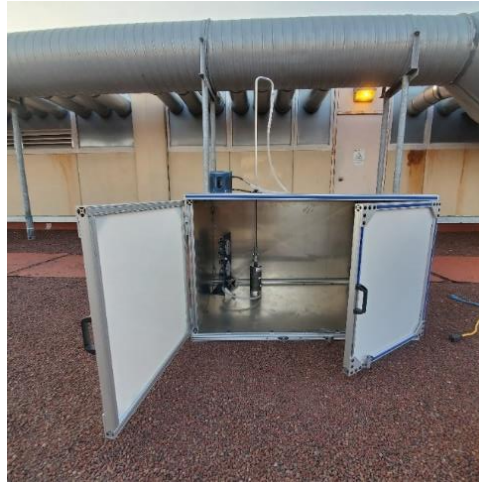
Figure 1.7: MOUDI was stored in an aluminum container for sampling during the wildfire.
