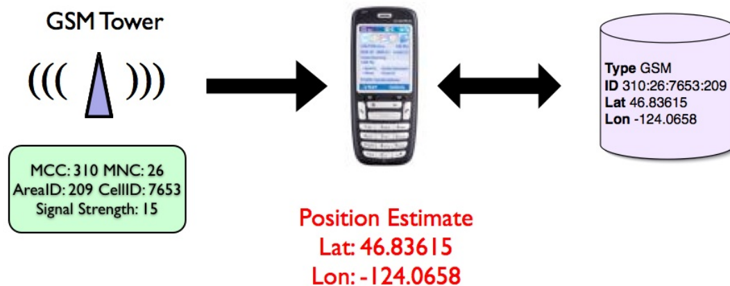
Figure 3.1: Overview of the Place Lab model. Mobile phones sense GSM towers (beacons) with unique ids. The phone uses the id to reference a beacon database. If the beacon is known, the phone estimates its position using the position of the beacons.
