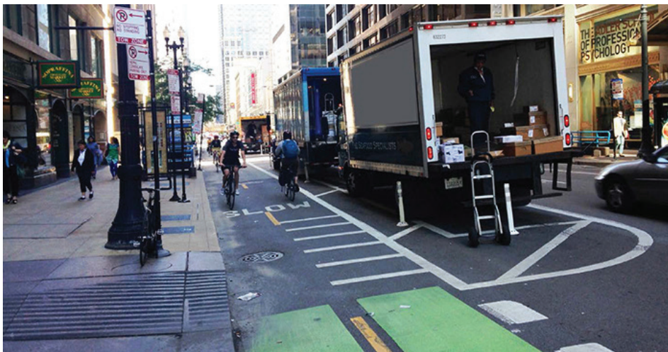
Figure 19. Delivery trucks in a “floating” parking zone along a protected bike pane in Chicago, II
