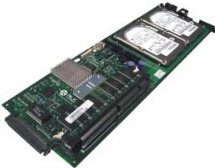
Figure 15 Typical Blade server Source: RLX Technologies
