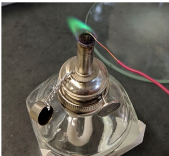
Figure 1: Image of positive Beilstein Test on a sample from the Resin Kit.
