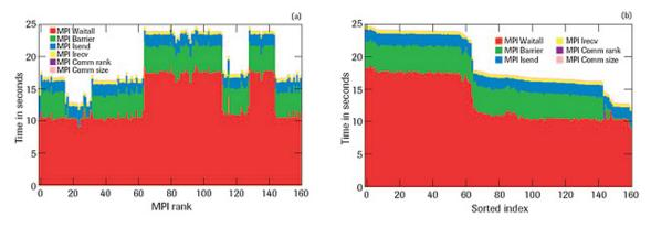
Figure 16. IPM can graphically present a wide range of data, including communication balance by task, sorted by (a) MPI rank or (b) MPI time.
