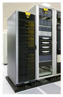
Figure 13. DaVinci is a 32processor SGI Altix with 6 GB of memory per processor and 25 TB of disk memory, a configuration designed for data-intensive analysis and interactive visualization.
