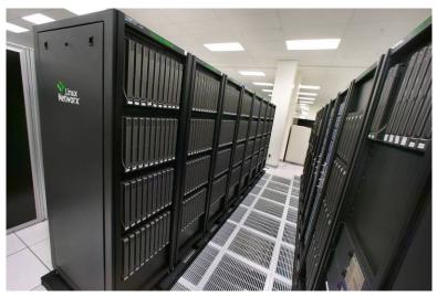
Figure 11. Jacquard is a 722-processor Linux Networx Evolocity cluster system with a theoretical peak performance of 2.8 teraflop/s.
