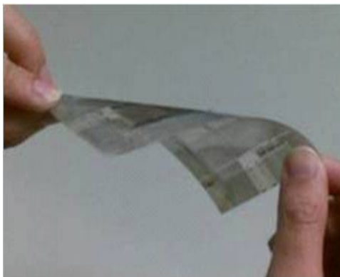
Figure 3.16: A device photo of transparent metal-oxide (IGZO) TFTs. (Photo courtesy of ITRI-FETD)
