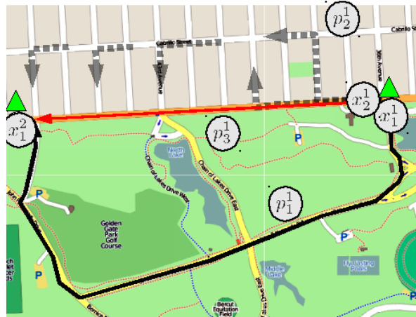
Figure 4-10: Example of a failure case when using a Hidden Markov Model: the solid black path will be favored over all the other paths.
