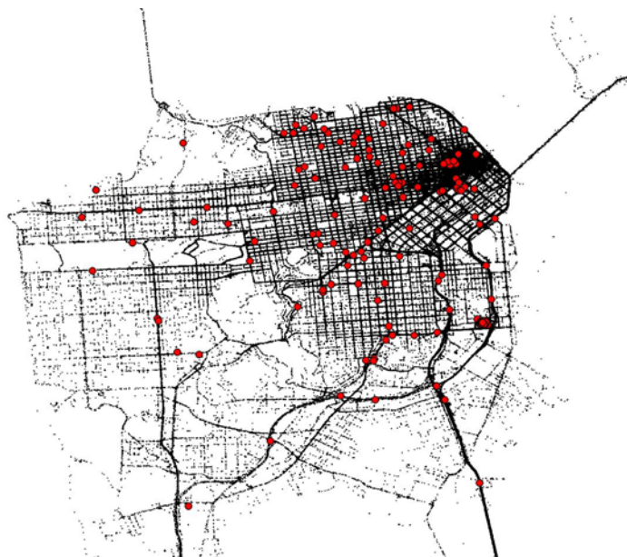
Figure 4-1: An example dataset available to Mobile Millennium and processed by the path inference filter: taxicabs in San Francisco from the Cabspotting program [22]. Large circles in red show the position of the taxis at a given time and small dots (in black) show past positions (during the last five hours) of the fleet. The position of each vehicle is observed every minute.
