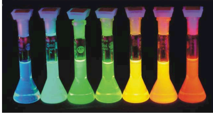
Figure 1.2: Quantum confinement effect in nanoparticles. Fluorescence of CdSe–CdS core–shell nanoparticles with a diameter of 1.7 nm (left, blue) up to 6 nm (right, red), giving evidence of the scaling of the semiconductor band gap with particle size. This image was adapted from reference (5).
