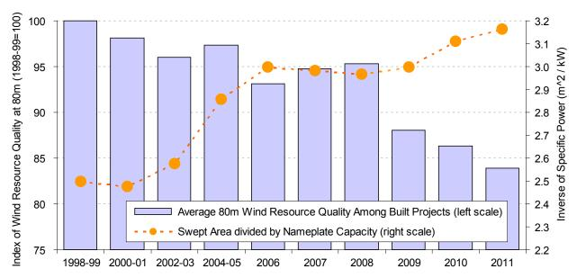
Figure 28. Index of Wind Resource Quality at 80 Meters vs. Inverse of Specific Power
