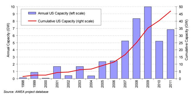
Figure 1. Annual and Cumulative Growth in U.S. Wind Power Capacity
