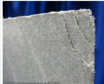
Detail of asbestos cement wall board
