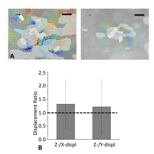
**Figure 2.5.** (A) Brightfield displacement map (with x- and y-displacements denoted by the direction and magnitude of the arrows, and z-displacements denoted by color) overlaid with shaded maps of displacement comparison. The white areas indicate regions where the x- and y-displacements exceed the z-displacements. (B) Overall, the z-displacements exceed both the x- and y-displacements (i.e. the displacement ratio is greater than 1).
