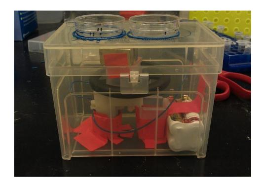
**Figure 3.1.** Magnetic actuator designed to reversibly induce a magnetic field to the coverslips. The battery-powered servo motor rotates the magnet alternatively between the two coverslip holders at ~60 RPM.
