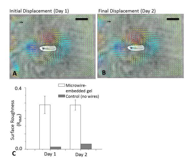
**Figure 2.9.** Topographical features are resistant to viscoelastic creep. (**A**) Initial displacement field induced by a microwire in a magnetic field, t=0 h. Scale bar = 20  $\mu$ m. (**B**) Displacement field after 20 h exposure to magnetic field; the displacement fields of (A) and (B) show no loss of features to viscoelastic creep. (**C**) TFM microscopy analysis shows no change in surface roughness over time (n=3).
