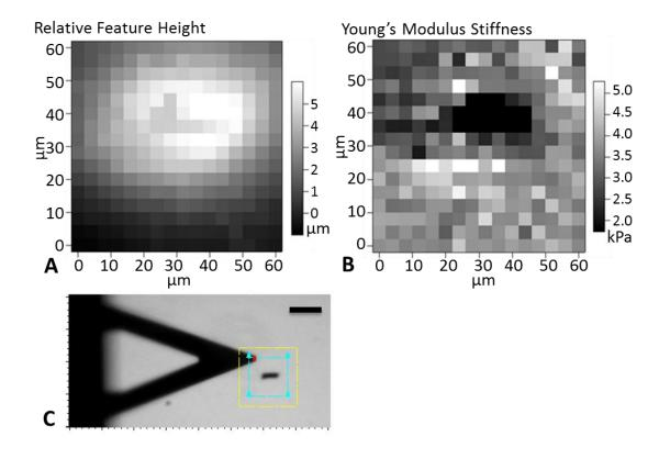
**Figure 2.8.** Effects of microwires on PA polymerization (**A**) Relative surface topography of hydrogel over a wire (**B**) PA stiffness decreases 2-fold over a microwire (**C**) Brightfield image of AFM scan. Yellow box outlines the maximum scan area; blue box outlines the scan area used  $(60\mu m \times 50\mu m)$ . Scale bar =  $50 \mu m$ .
