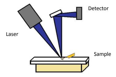
**Figure 2.6.** Schematic of AFM mechanism. A laser is directed at the pyramidal cantilever tip, which then deflects light to a point on the detector. When the cantilever tip indents into the sample, it bends slightly and changes the position of the deflection beam.
