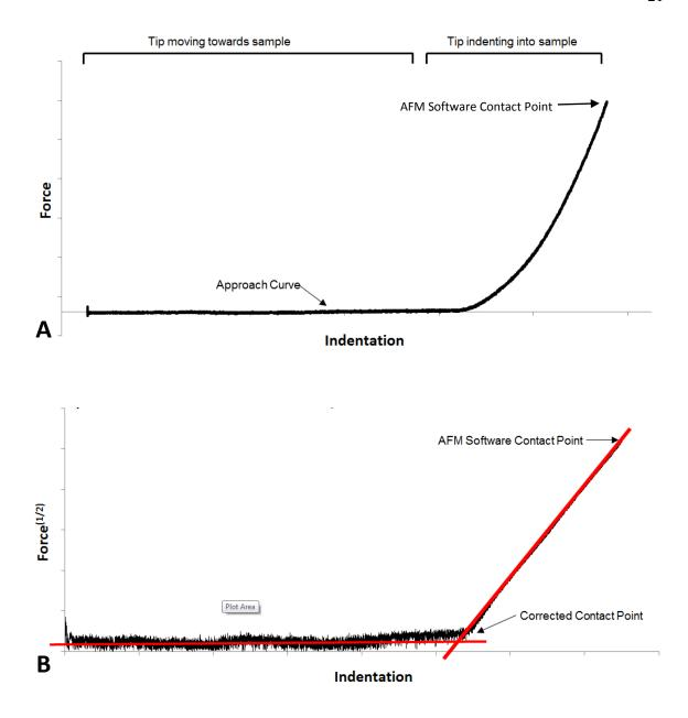
**Figure 2.7.** (A) AFM force curve and corresponding (B) Hertzian transformation highlighting the two linear regions and corrected contact point.
