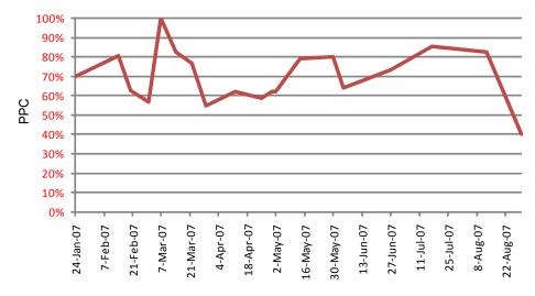
Figure 4.3: Percent Plan Complete (PPC) figures for a portion of the project.
