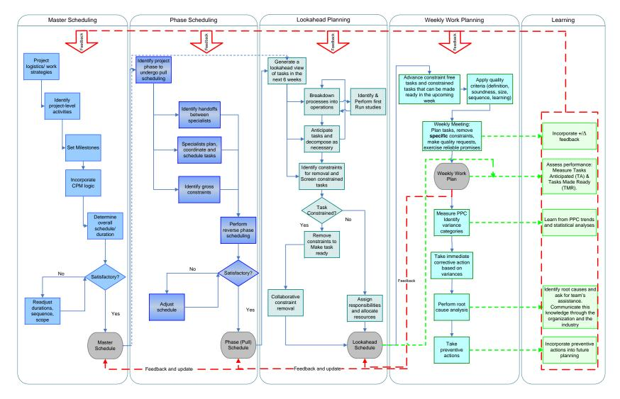
Figure 5.3: The Last Planner<sup>TM</sup> System (adopted from Ballard and Hamzeh 2007)
