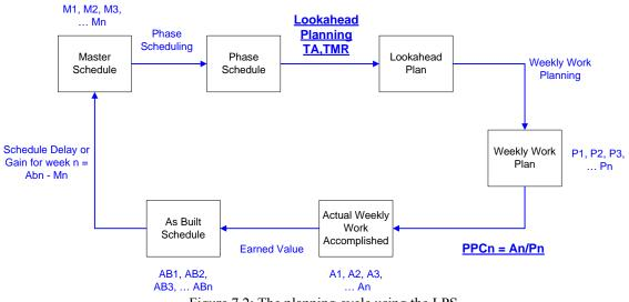
Figure 7.2: The planning cycle using the LPS.
