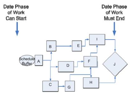
Figure 5.10: Reverse phase schedule adjusted to create a schedule buffer (Ballard 2008)
