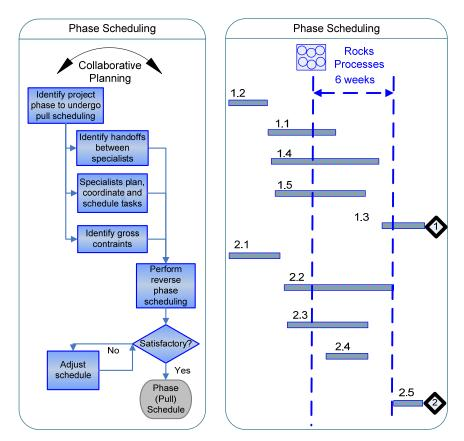
Figure 5.8: The phase scheduling process in the LPS
