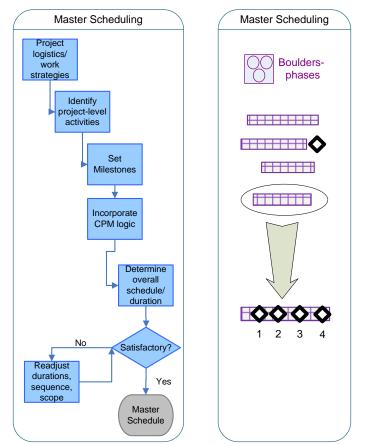
Figure 5.7: The master scheduling process in the LPS
