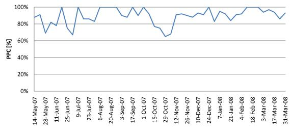
Figure 1.2: Percent Plan Complete (PPC) tracked over time.
