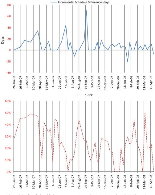
Figure 4.4: The relationship between percentage of work not complete (1-PPC) and incremental schedule difference for building '601'
