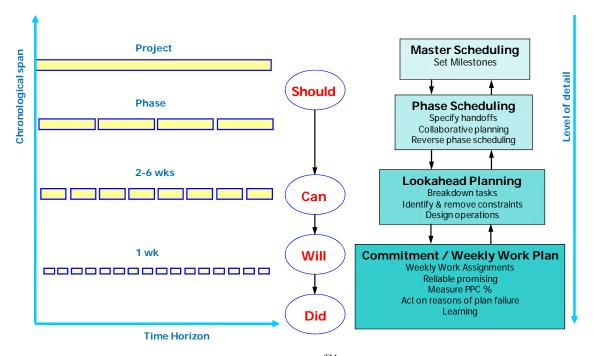
Figure 5.2: Planning stages/levels in the Last Planner <sup>TM</sup> system for production planning and control (Adjusted from Ballard 2000a).
