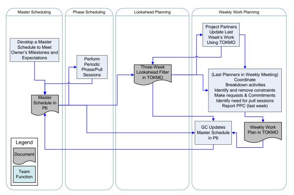
Figure 4.7: Implementing the LPS on UCSF's CVRC
