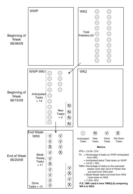
Figure 5.14: Measuring tasks anticipated (TA), tasks made ready (TMR), and percent plan complete
