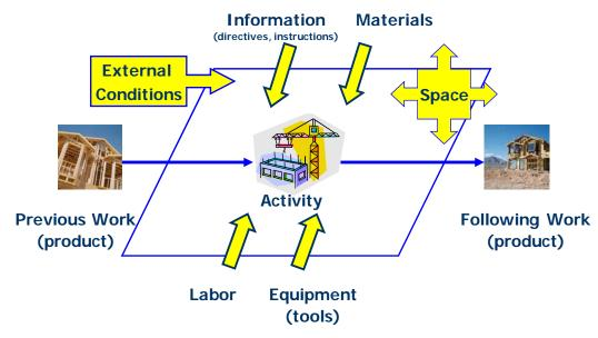
Figure 2.1: Flows involved in a construction activity; after Koskela (2000).
