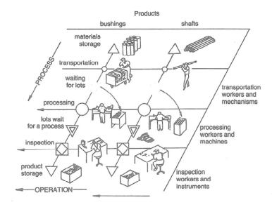
Figure 2.4: Flow of process and operations (Shingo 1988).
