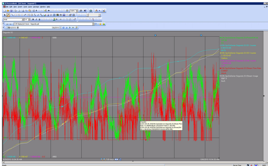
Figure 6. View of PI Processbook (Realtime Data View). Legends from the top are 1) total kW (green), 2) cumulative counter for BTU/h (blue), 3) cumulative counter for gallons of water (yellow), 4) klbs/h of steam flow rate (red), 5) lbs/h of steam usage (white)
