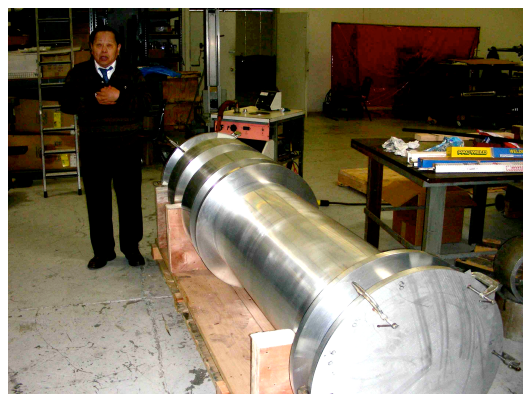
Fig. 1. The Magnet Forged 6061-T6 Mandrel during Machining.
