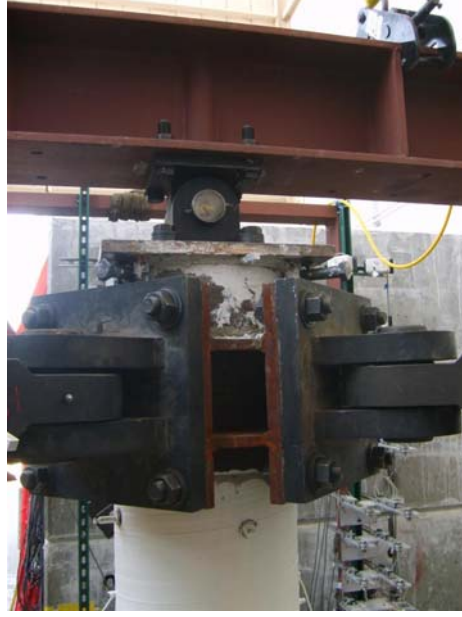
Fig. C.9 Attachment of actuators to the column
