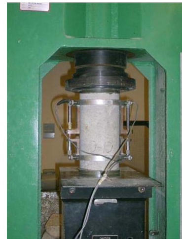
(b) Compression test
