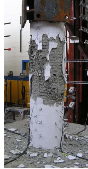
(b) Axial failure of the column
