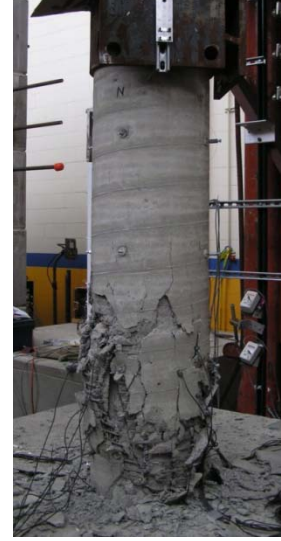
(b) Axial failure of the column
