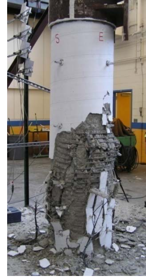
(b) Axial failure of the column
