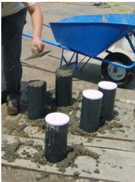
(a) Casting concrete cylinders
