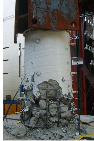
(b) Axial failure of the column
