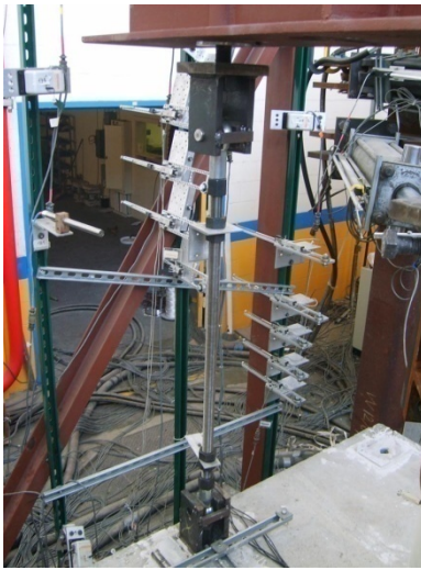
(a) Post-tensioned rod
