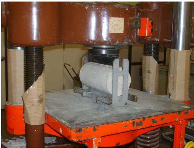
(a) Splitting test
