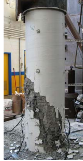
(b) Axial failure of the column
