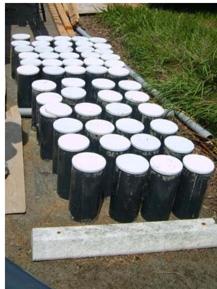
(b) After casting concrete cylinders
