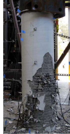
(b) Axial failure of the column
