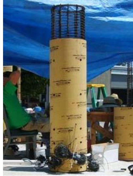
(b) After putting the Sonotube
