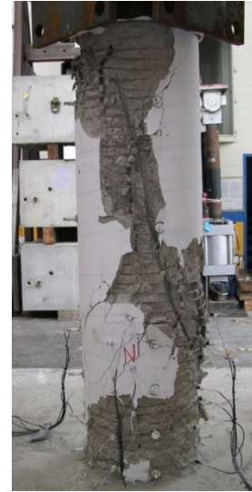
(b) Axial failure of the column
