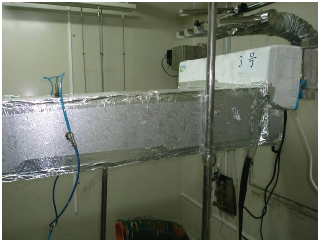
Figure 8 Air Enthalpy Method at Laboratory 2
