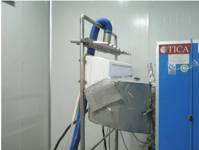
Figure 9 Air Enthalpy Method at Laboratory 3
