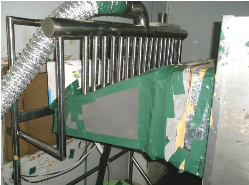
Figure 6 Air Enthalpy Method at Laboratory 1
