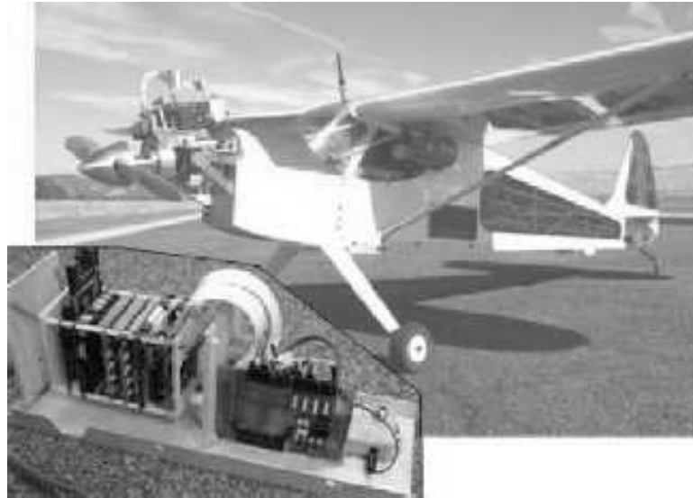
Figure 7.5: Sig Rascal 110 UAV and a single PC-104 stack
