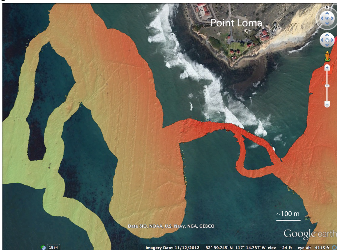
Figure C-8: Multibeam bathymetry offshore Point Loma collected in 2012 using a Reson 7125 system operated at 400kHz and with real-time kinematic navigation. Grid resolution is 0.5 m. Dipping beds represent the Cretaceous Rosario group, which makes up much of the substrate beneath the Point Loma kelp forest.
