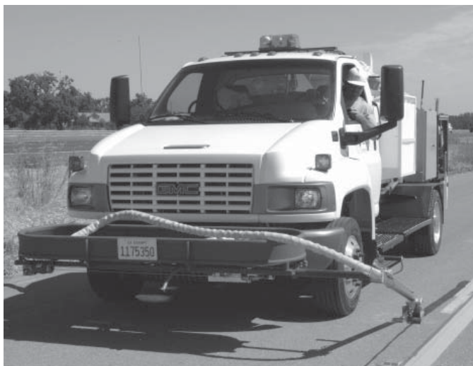
The Sealzall multipurpose crack sealer, developed by the AHMCT's Duane Bennett. The driver controls the machine by remote control.
