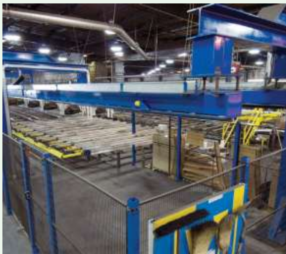
Figure 6. Kaiser Aluminum's Sherman plant operates three extrusion press lines like the one pictured above, which convert aluminum scrap and ingot into aluminum extrusions.
