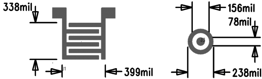
Figure 4.3: Simple capacitive electrodes fabricated on Kapton.
