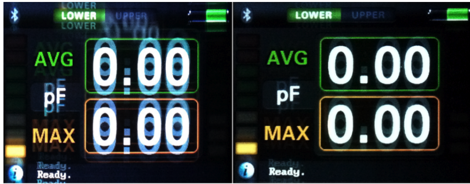
Figure 7.11: Large reduction in glare with the application of a polarizer film.
