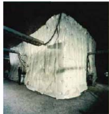
Figure 13. Schematic three-dimensional perspective of the SHT [Tsang et al., 2009] and photo of single heater test block insulated [Wang and Bodvarsson, 2003].
