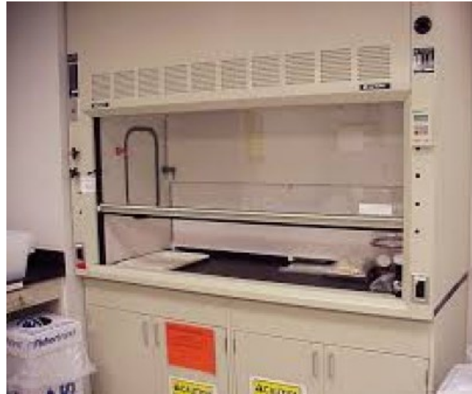
When at the lab I will remember to press the fume hood down completely when not in use.
