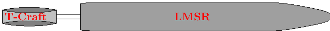
Figure 4.4: Top view of a bow to stern configuration. Bow of an SES is connected to stern of an LMSR by a ramp.
