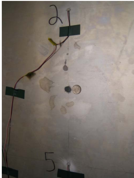
Figure 4.7. Picture of salt water corrosion spots around damage 1.
