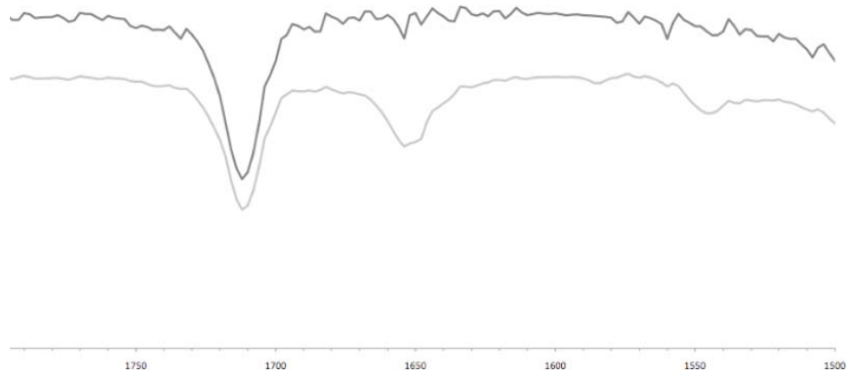
Figure 4-13. Infrared spectroscopy (IR) of 25:1 Leu NTA: nickel initiator at 80 °C in the absence (dark purple line) and presence (light purple line) of 10 mol % \text{Fe}(\text{CO})_3(\text{PPh}_3)_2
