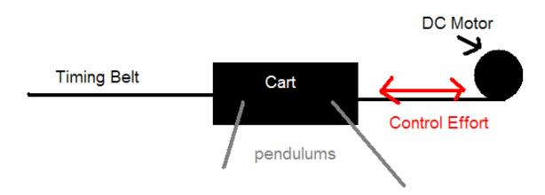
Figure 1: Diagram from original dual inverted pendulum swing up test stand.
