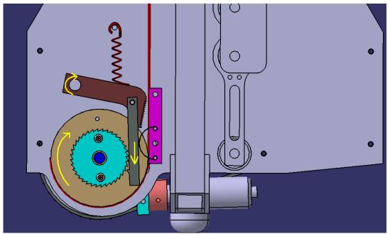
Figure 24: Tan Pulley is rotated clockwise causing the dark grey pawl to move down, which in turn rotates the brown cam clockwise causing the rope to disengage from the cam.
