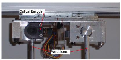
Figure 7: Cart Mounted to Ecoline Slider
