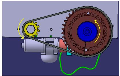
Figure 27: The Blue motor housing (which is attached to the orange pulley, which is fixed to the brown sprocket) is turned counterclockwise which turns the yellow sprocket counterclockwise via a chain.
