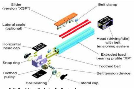
Figure 5: Rollon Linear Evolution Ecoline track
