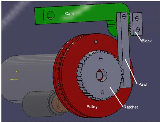
Figure 13: Iteration 2 for quick release mechanism: Masterclam 3001 (front isometric view)
