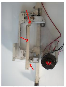
Figure 19: An additional 4-bar-linkage was added in an attempt to counteract lock mode. Red arrows indicate the new members added
