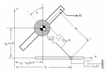
Figure 39: I-hop Equations of motion Diagram
