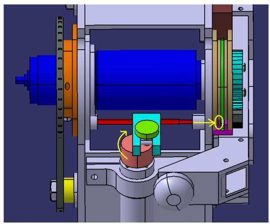
Figure 26: The salmon pink clutch pulley turned as shown clutch pin to be pushed through the tan pulley. This locks the shaft of the motor to the housing of the robot.
