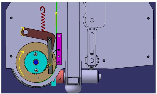
Figure 29: The Tan pulley is turned clockwise which pulls the dark grey pawl down. This motion turns the brown cam clockwise which disengages the cam action on the rope-spring. When the cam is disengaged the slack in the rope is freed quickly.
