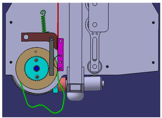
Figure 25: The tan pulley is rotated counterclockwise, which allows the dark grey pawl to move up. This action causes the brown cam to be rotated counterclockwise which engages it onto the rope.
