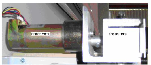
Figure 6: Linking Pittman motor with optical encoding with Ecoline track's "Toothed pulley"
