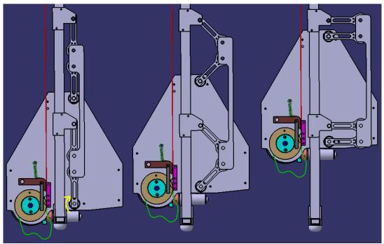
Figure 28: The yellow sprocket is attached to the bottom link of the coupled four bar linkage causing it to unlock. Once the coupled four bar linkage is unlocked the energy stored in the red rope-spring is then used to drive the pogo assembly down as shown.
