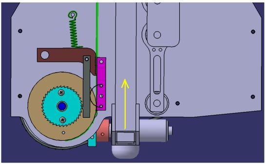
Figure 30: With no rope spring to resist motion of the pogo assembly it is easily pushed back into place my the force of the landing robot.
