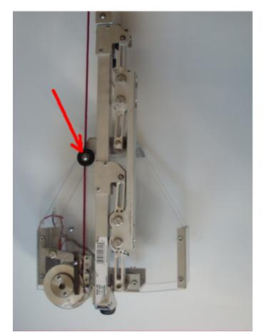
Figure 21: Implementation of one bearing to try to keep the pogo assembly straight
