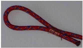
Figure 12: Spectra Core Rope Bound with copper wire
