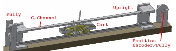
Figure 2: Overview of CAD model for undergraduate dual inverted pendulum test stand
