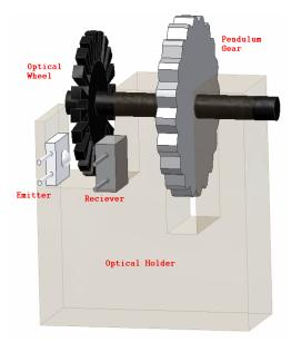
Figure 4: Close up of wireless mouse encoder used for transmitting pendulum angle to the computer for undergraduate dual inverted pendulum test stand.
