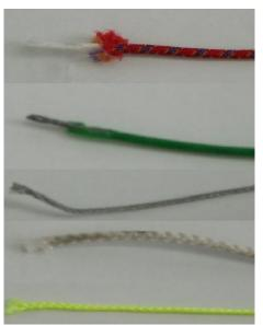
Figure 11: Rope Tests: (from top to bottom) Spectra Core rope, Poly Vinyl coated steel cable, Steel cable, Braided nylon rope with core, Nylon rope
