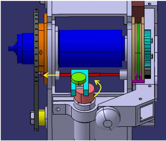
Figure 23: Salmon clutch pulley forces the green pin to push the aqua fork that is attached to the red clutch pin to lock the orange pulley in place. This action is made possible by the small motor driving the pink clutch pulley until the green pin hits the grey pin causing the motor to stall. This locks the housing of the motor to the housing of the robot.
