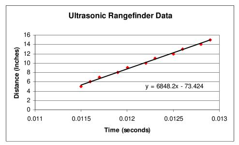
Figure 42: Finding Bias for Ultrasonic Rangefinder
